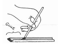
3. Press channel to rib of board. Start at one end as shown.
