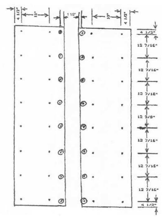
5 Sheets of plywood 4'x8' 5/8" thick to be cut in half to make 10 sheets 2'x8'
