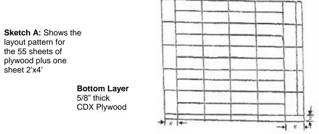
Requires: 55 Sheets of plywood 4'x8' 1/2" thick and 1 sheet 2'x4' 1/2" thick With 5 sheets to be cut in half to make 10 sheets 2'x8'
